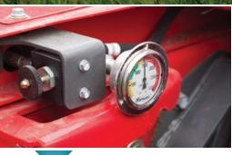
Hydraulic conditioning roll tension on the 1393 & 1316S. This is the first pull-type design to have this system.
