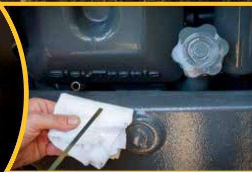
Engine oil can be checked and topped from ground level
