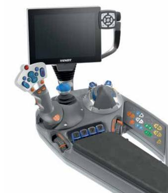
The complete controls for the tractor are integrated into the multi-function armrest, which is attached to the seat.
