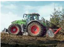
When working in reverse-drive mode, all control elements can be operated just as comfortably as in front-drive mode. The entire driver station can turn 180°— and everything else in the cab remains where it is.
