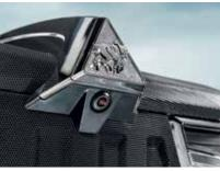
Practical for front-mounted implements, the new camera integrated in the hood captures the view to the lower links and transmits the image to the Varioterminal.
