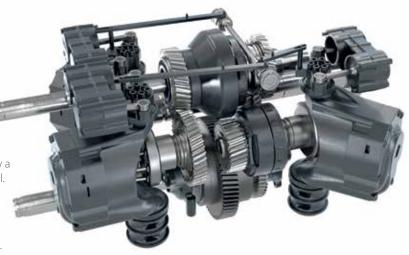
New, larger high-capacity hydrostats with 22.6 in<sup>3</sup>. provide greater transmission efficiency.
