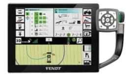
The Variotronic<sup>11</sup> headland management system allows the operator to save all the procedures used when performing a specific maneuver. Variotronic<sup>11</sup> automatically triggers the sequences at precisely the right place.
