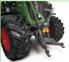
Standard 40-GPM hydraulic system with optional 54-GPM independent hydraulic pump with up to 6 rear and 2 front hydraulic valves; single and double acting front 3-point options give you the right configuration for any application.
