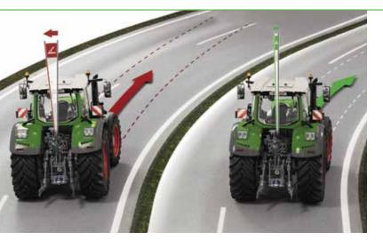
Optional Fendt Stability Control (FSC) takes steering precision, driving stability and braking safety to new levels. At speeds above 12.4 mph (20 km/h), FSC locks the front axle suspension cylinders and dampens side-to-side movement to ensure maximum stability in transport. When speeds drop below the FSC threshold, it automatically disengages to ensure maximum ground
