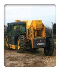
**FRAME TILT** up to 10° to the left and right to increase stability on steep or uneven terrain.
