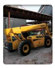
LOW MACHINE HEIGHT allows easy passage under 8 foot (2438 mm) doorways.
