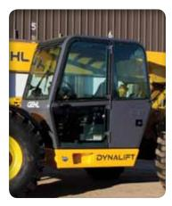
**CAB OPTIONS** in an open canopy for mild climates and rental applications or enclosed with heater and defroster. Air-conditioning is optional on the enclosed cab models.
