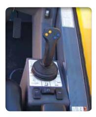
**CONTROL OPTIONS** include a single joystick with dual-function or tri-function operation. The dual-function joystick allows for proportional control of attachments and auxiliary hydraulics.
