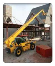
EXCELLENT HYDRAULICS rated at 43 gpm (163 L/min) for smooth control function and extra power to operate a variety of attachments.
