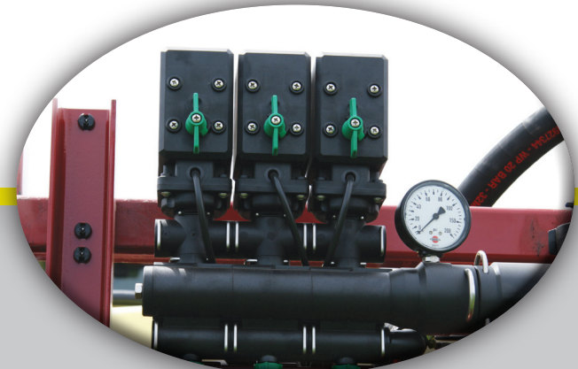
EVC Control 3 section with constant pressure.
