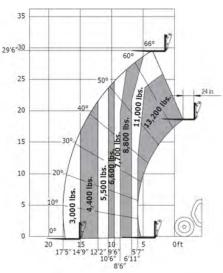
Load chart based on 24 inch (600 mm) load center per ANSI B56.6.
