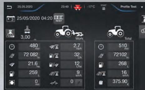
► **Memorize data and settings** — An unlimited number of user setting configurations enable the system to record information during operation on area worked, fuel use, hours worked and much more. All the settings and parameters can be stored by the Datatronic 5 terminal and recalled to find a previous setting.
