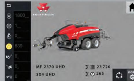
► **ISOBUS for total implement control** — ISOBUS allows an implement manufacturer's control system to be displayed on the terminal screen, saving owners and operators time and money, with no need to install additional monitors in the cab. Simply plug the implement lead into the tractor's ISOBUS socket and the system automatically uploads the operating menus and displays on the screen.
