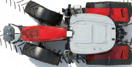
▼ **SPEEDSTEER** reduces operator effort and provides faster turns, maximizing your time in the cab. It enables the operator to adjust the steering ratio and select the number of turns of the steering wheel required for a given amount of steering angle turns.
