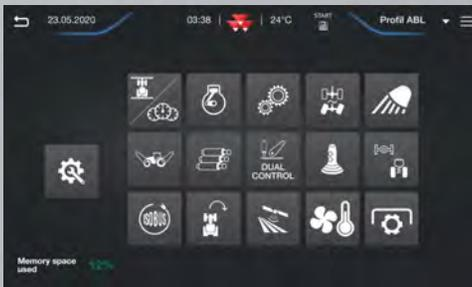
► **Full tractor function management** and optimization features for transmission, engine and hydraulics. The Dual Control system provides excellent control of semi-mounted plows by automating the furrow entry and exit. At the same time the system adjusts the plow's depth wheel in relation to the rear linkage.
