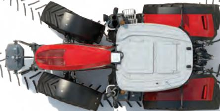
▼ **SPEEDSTEER** reduces operator effort and provides faster turns, maximizing your time in the cab. It enables the operator to adjust the steering ratio and select the number of turns of the steering wheel required for a given amount of steering angle turns.
