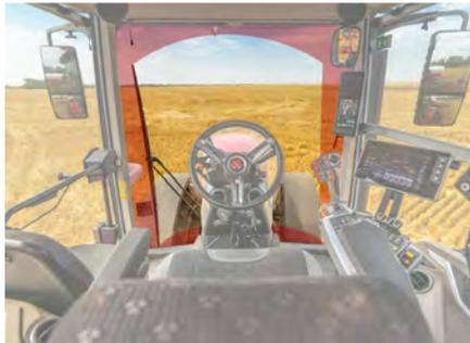
**SIDE MIRRORS** feature an adjustable top and lower section offering the best view during transport and reducing blind spots. Options include electric de-icing and electronically adjustable mirrors.
