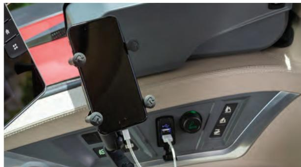
**ALWAYS CONNECTED** — Two USB ports and adjustable phone and tablet holder available through AGCO Parts.
