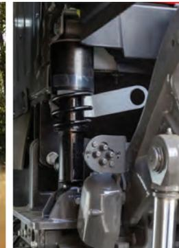
**CAB SUSPENSION** brings extra comfort. Two types available: mechanical and active mechanical.
