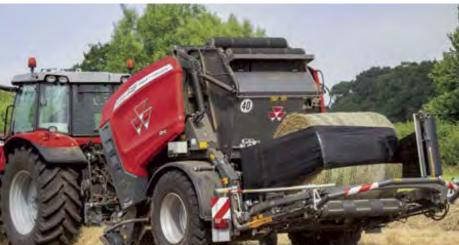
Once the bale is transferred to the center of the wrapping table, a hydraulically driven wrapping ring begins to rotate before the tailgate is fully closed, completing the cycle well before the next bale is ready to wrap. Designed to withstand the heaviest bale loads, the robust frame and quiet running gear operates smoothly and effortlessly to wrap bale after bale.
