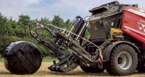
To ensure gentle bale unloading, the wrapping table is lowered close to the ground, thus minimizing the bale's rolling speed, preventing film damage and maintaining the ideal bale shape. An optional bale tipper prevents bales rolling away and makes for easier trailer loading. The operator can also choose between automatic and manual unloading modes.
