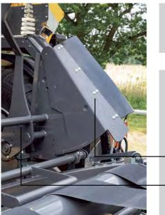
The new Protec combination unit has a lower crop elevation angle, reducing the overall baler height. This feature improves stability, allowing safer and faster hillside operation. It also reduces back pressure in the feeding area, streamlining crop flow and minimizing the risk of blockages.
