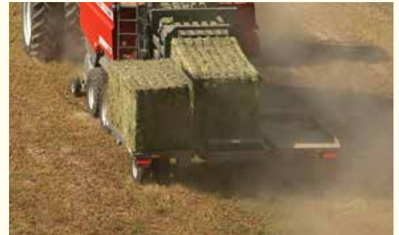
Large bale accumulators collect and group bales in the field.
